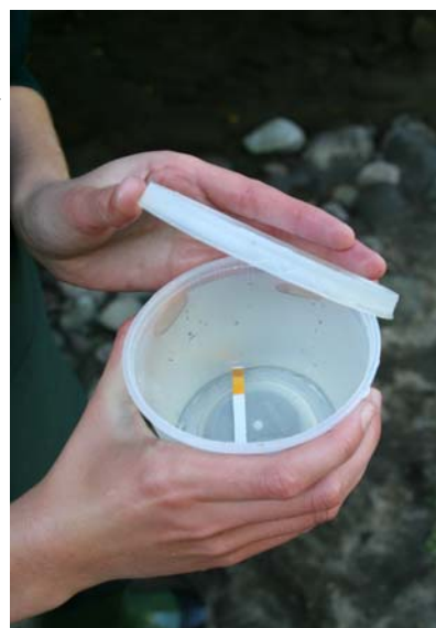
Figure 4 Measuring water pH with ‘Merck Neutralit’ pH strips.
