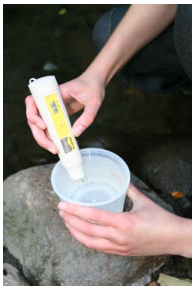
Figure 3 Measuring water conductivity with the ‘EUTECH Cybernetics TDScan 3’ conductivity instrument.
